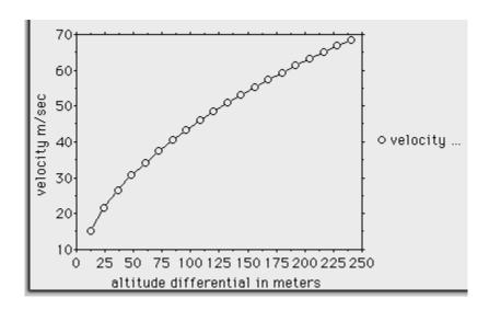
We see that the curve of velocity at first increases more steeply and then tends to flatten with higher altitude differentials.
