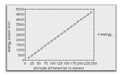
The increase of energy output is linear, as shown in the graphic above.
