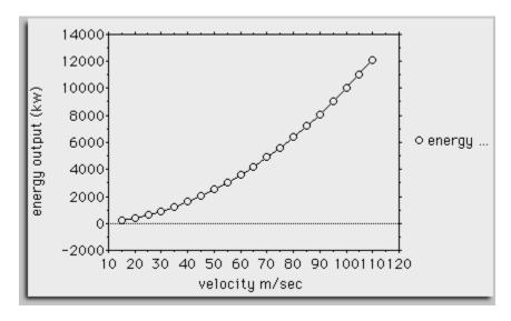
The graphic representation makes it clear, that a velocity increase brings progressively larger increases of energy. Therefore, the higher the velocity of the water, the greater the overall efficiency of the power plant!
